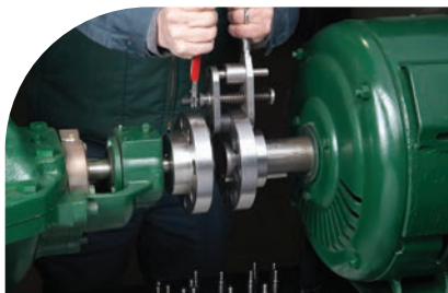
Installation of bushings using tool and ratchet wrench
