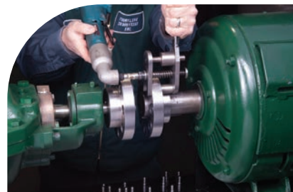
Removal of bushing using tool and angle ratchet wrench
