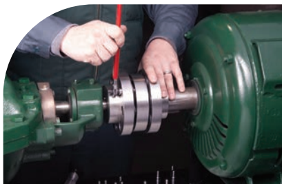
Installation of pins using ratchet wrench
