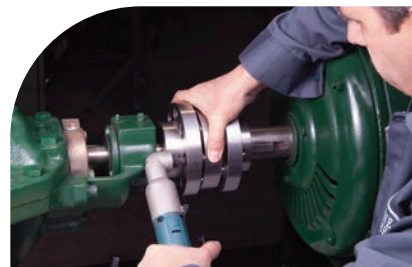
Final torquing of pins
