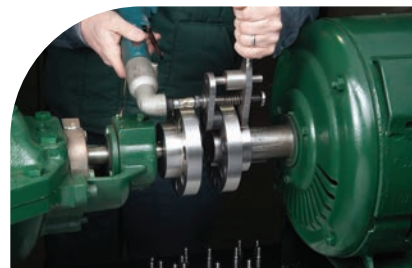
Installation of bushings using tool and battery operated angle ratchet wrench
