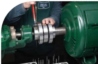
Removal of pins with ratchet
