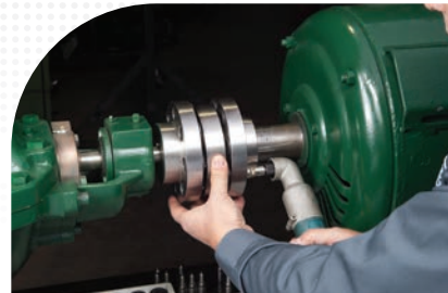
Removal of pins with cordless angle ratchet wrench
