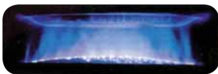
Axial Magnetic Field Interrupter - Arc Dispersion
